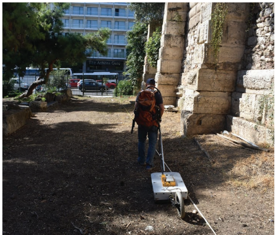
Fig. 1: Ground penetrating radar survey using a 250 MHz antenna southwest of the main wall of the Olympieion.
